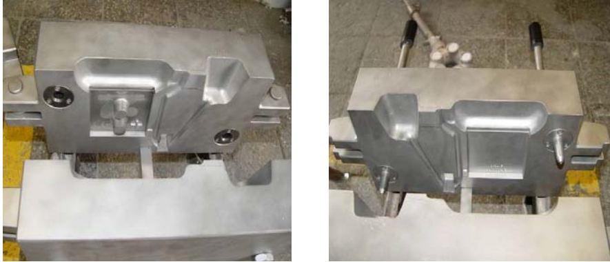
Fig. 1 Design of permanent metal mould
